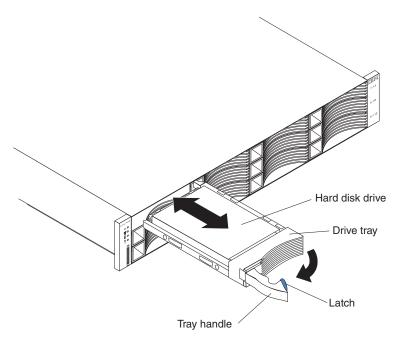
Figure 47. Installing and removing a hard disk drive
